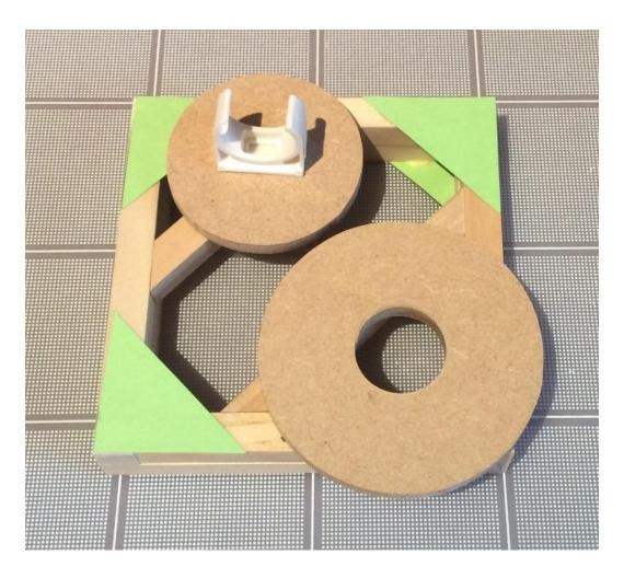
Assemble the model as shown and then push the tubing onto the syringe tip. To operate the platform, attach the other syringe with its plunger out onto the tubing; then push its plunger in.
