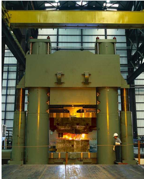
Figure 1.2.: 40,000 ton forging press. Source: Shultz Steel.
