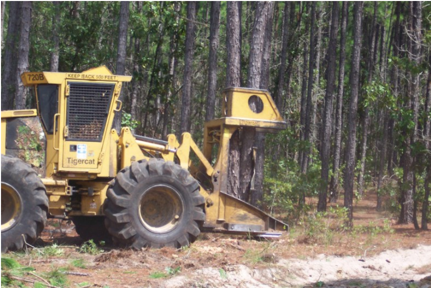
Figure 1.5.: Feller buncher. Souce: Wikipedia image.
