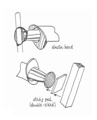
Using an elastic band and a stirrer or popsicle stick is a useful way of lining things up temporarily.
