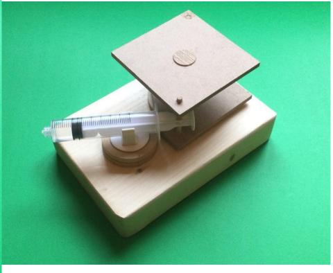
Close the piston-syringe on the structure and then attach the other piston-syringe, fully open, using the length of tubing.
