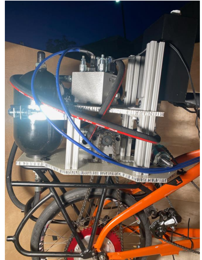
Double-deck design with composite mounting panels
