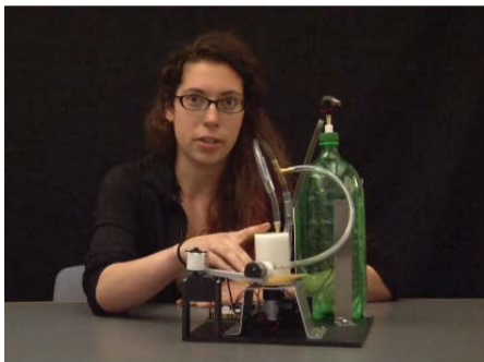
Figure 4. Some examples of student use of pneumatics. Left to right: Lauren Kuntz and her custom valve. Katie Gero’s centrifugal pump. Daisy Yuen’s positive displacement pump.
